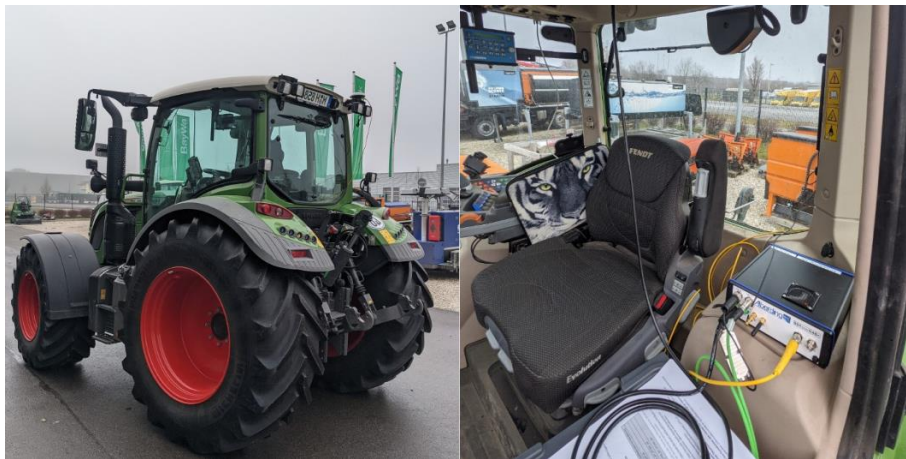
Field trials of the A10 DAB+ sensor in the agricultural sector demonstrated the reliable use of PPP RTK transmission via DAB+. (© Alberding GmbH)
