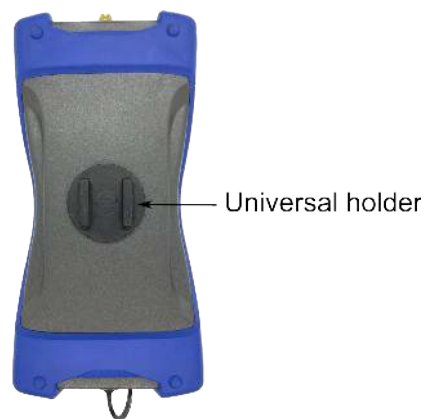
Figure 4: Back side with universal holder
