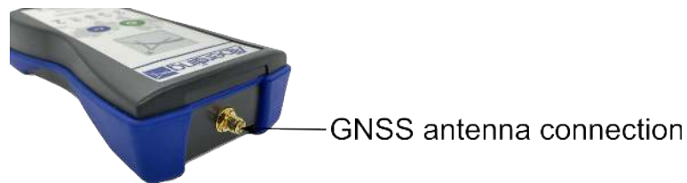
Figure 2: GNSS antenna connection
